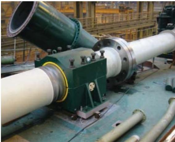
New Composite cutterhead intermediate lineshaft bearing installed
