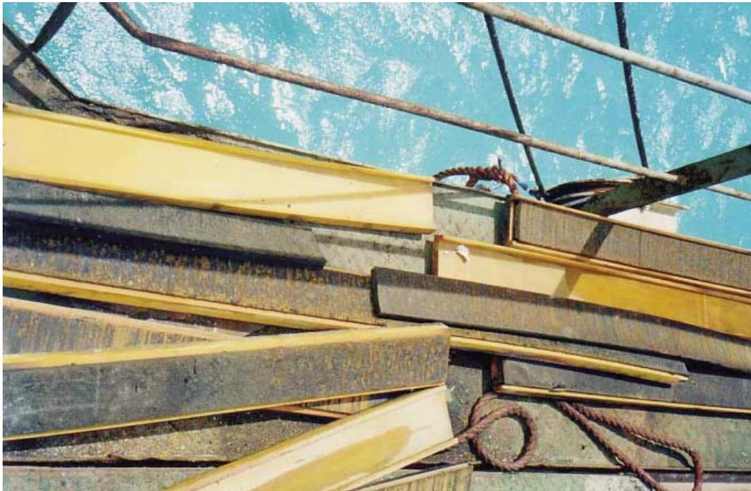
*Thordon Composite staves originally installed in February 1996 were removed after over five years of operation*
