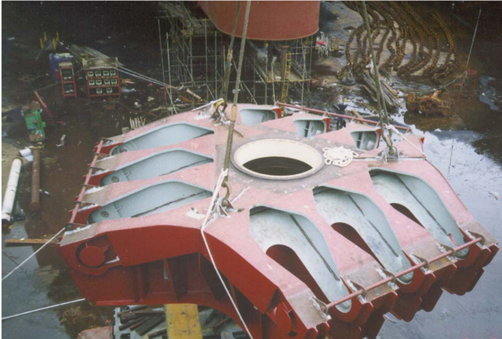
Bow turret of Ruby Princess prior to installation
