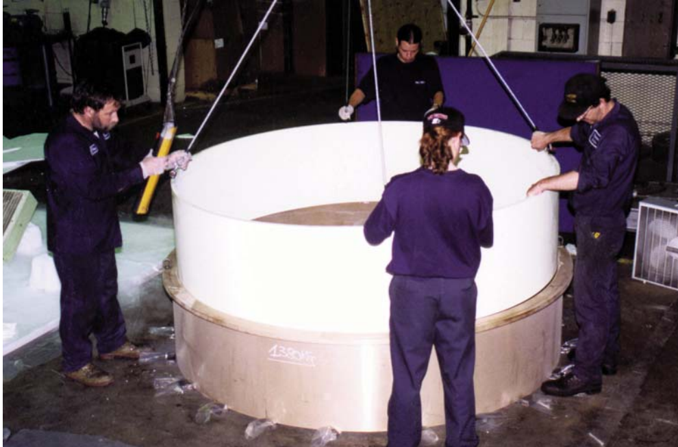
Installing SXL into bronze carrier
