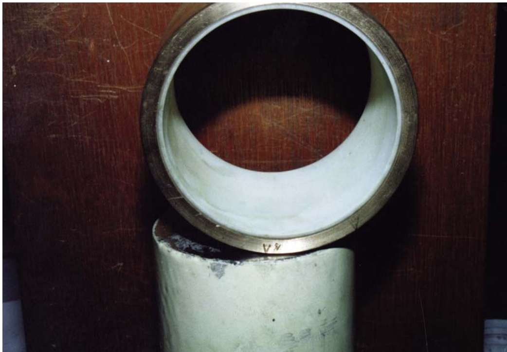
Test bearing and spool after 38,000 test cycles
