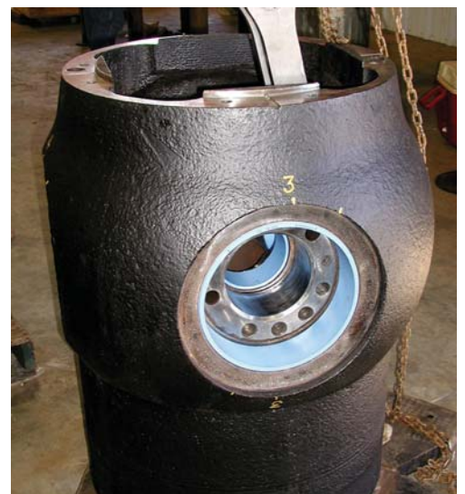
Alabama Electric installed ThorPlas® runner blade trunnion bushings for their Kaplan turbine
