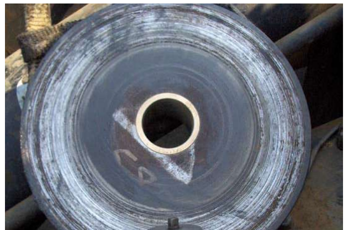
HPSXL TRAXL bearings installed in Kronos truck pulley
