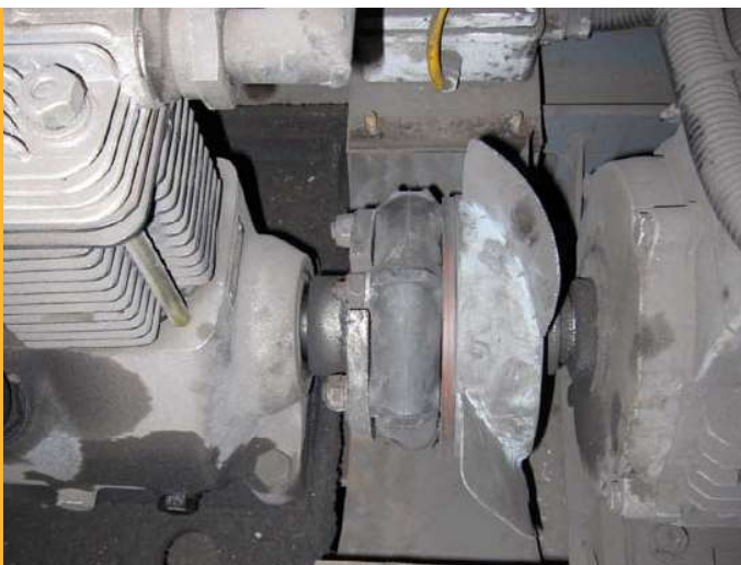
MUTC public trolley bus hardy clutch system
