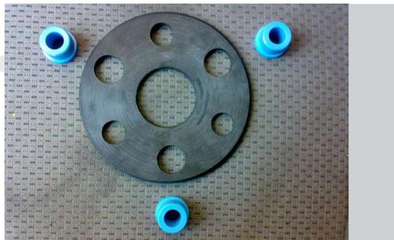
Replacement of clutch Tecamid parts with ThorPlas-Blue
